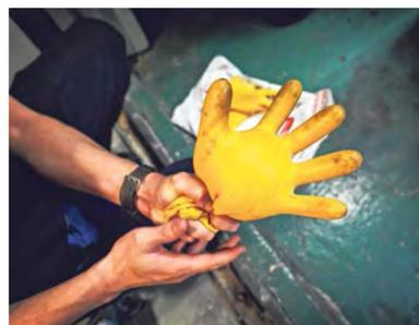
Technician Mohd Iskandar Mohamad Sopi inflating a high-voltage glove to check it for tears or leaks before putting it on. This insulated glove, part of his personal protection equipment, prevents accidental electrocution on the job. Lifts are run on voltages of up to 400 volts and currents of up to 40 amps.
