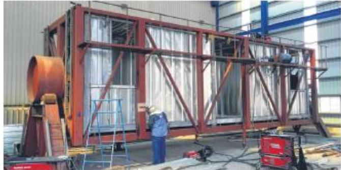
1. Each time, 40-50 empty modules manufactured in prefabrication plants in China are shipped to Singapore. They have floor tiles, windows, internal door frames and internal boards installed.
