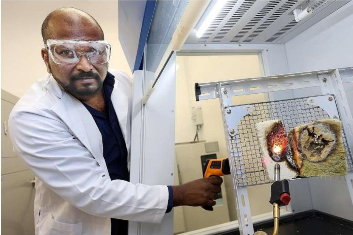
Dr Mahesh demonstrating the fire resistance of NTU's newly developed foam (left) over conventional insulating material (right) when put under a blowtorch flame at almost 2,000 deg C. NTU's innovation and enterprise arm NTUitive has filed a patent for the product. ST PHOTO: LAU FOOK KONG
